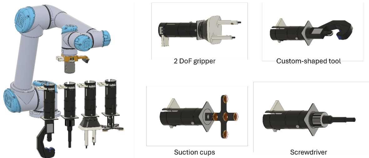
Figure 44: Schematic representation of the smart end-effector developed for the Campetella use case
